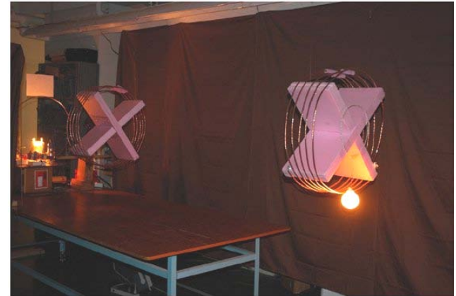
Fig. 2 Verification experiment model by MIT [2] The transmitting efficiency was 40% (Helical coil distance was 2.1 m).
